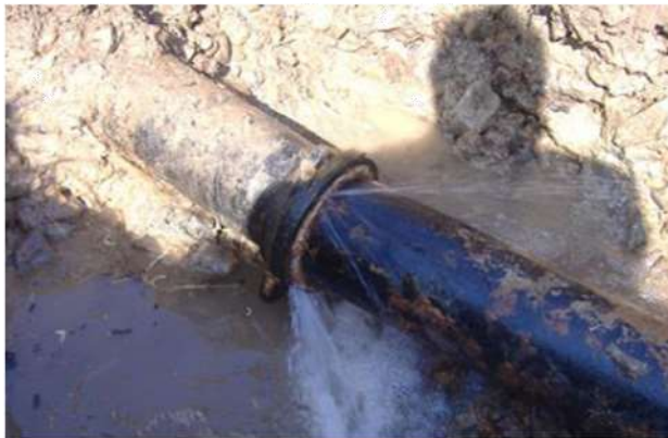
Figure 7-2: Cast Iron Pipe Failure
